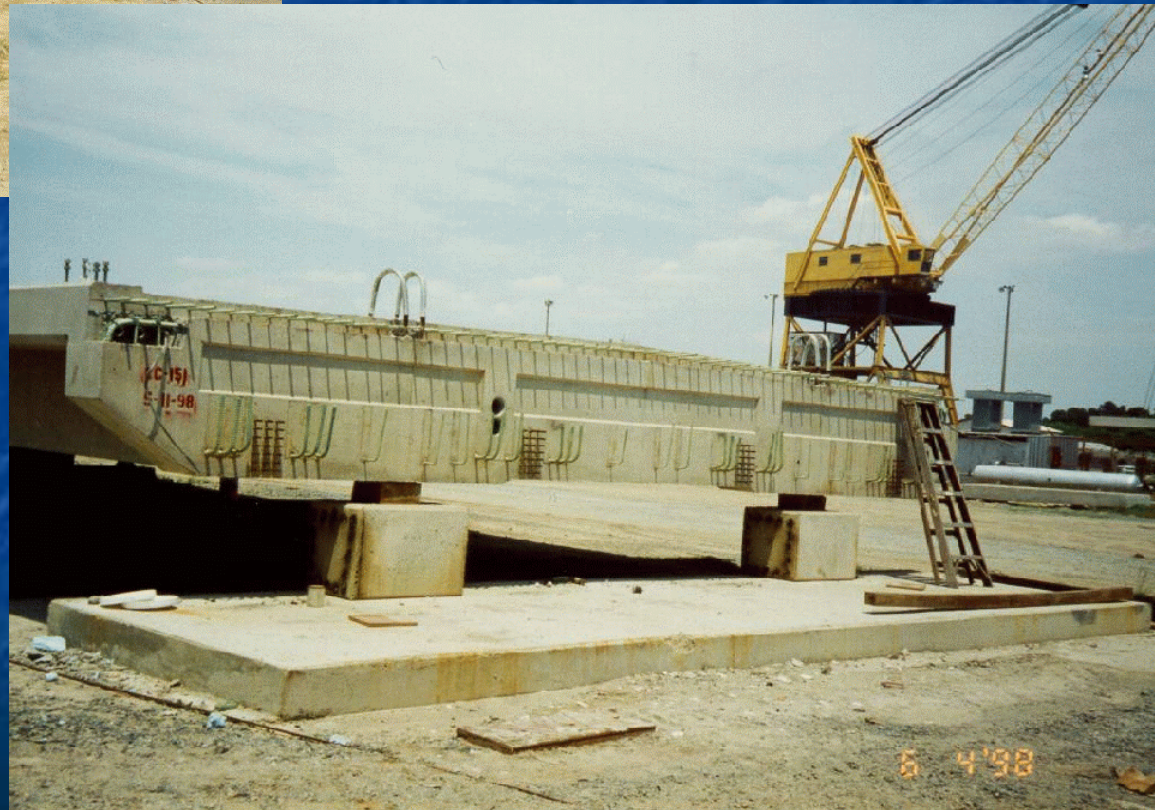
Quad-Tee full width deck segments at the precast plant
