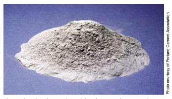
**Fig. 6**. Fly ash, a by-product of the electric industry, can be used as a partial replacement for portland cement.
