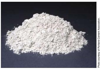
Fig. 7. Slag cement is a cementitious material and also a byproduct of the iron industry.
