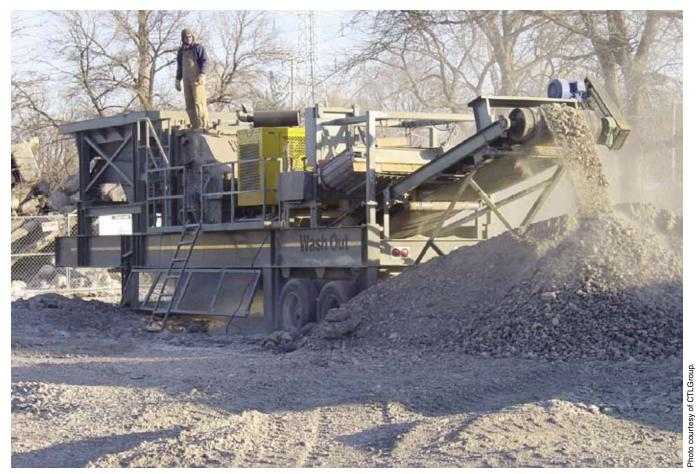
Fig. 9. Crushed concrete from other sources can serve as recycled aggregate.
