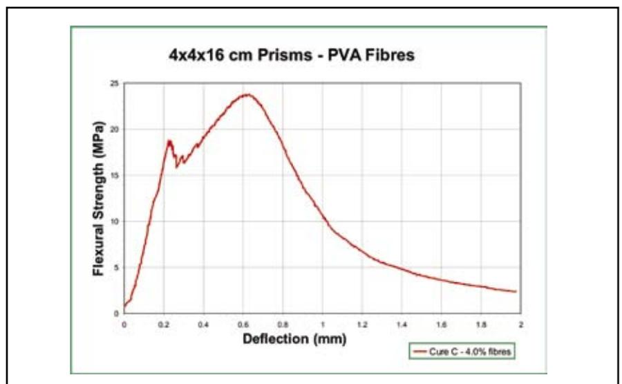
Fig. 3. Load-deflection curve for prism loaded in four-point bending.
