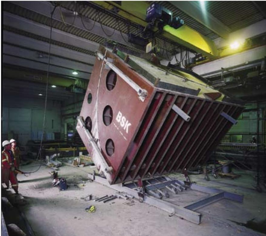
Fig. 12. The form is rotated 180 degrees to an upright position after the material gained enough strength. (Courtesy of Tucker Photo.)
