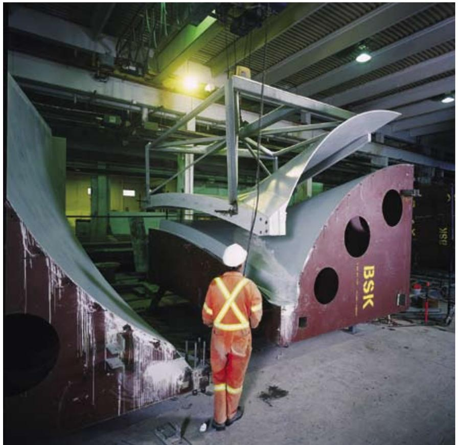
Fig. 14. Demolding of the precast canopy element. (Courtesy of Tucker Photo.)
