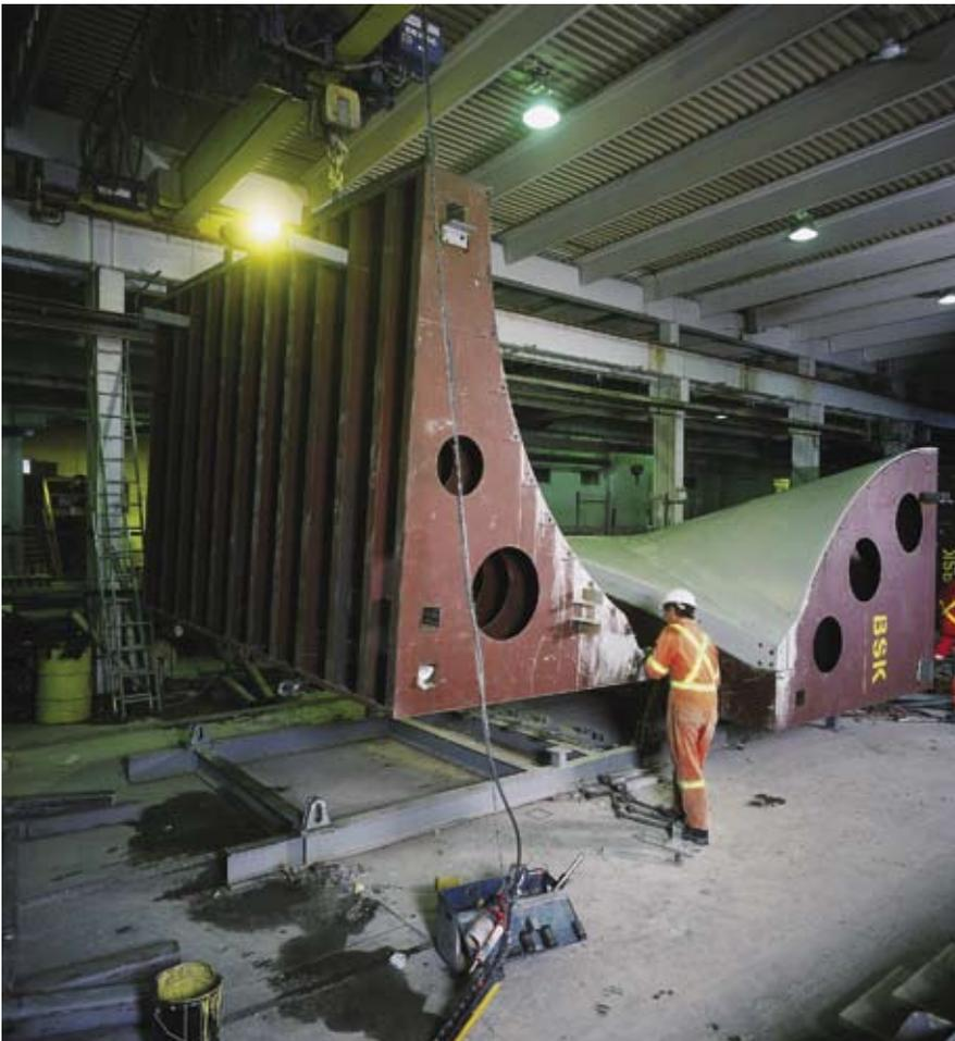
Fig. 13. Top form is lifted from mold. (Courtesy of Tucker Photo.)
